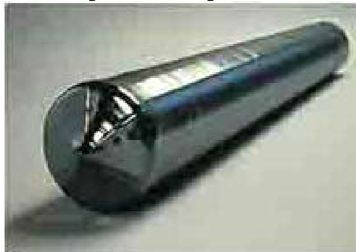
Monocrystal of semiconductor "solar" silicon
