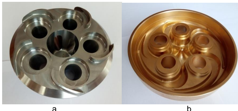
Figure 12. Experiment Sample of the Shell (a) and the Crown Tip (b) of the Oxygen Blowing Lance.
